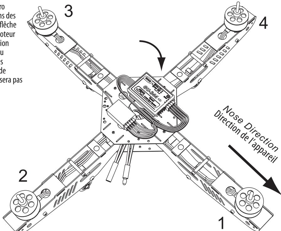
After checking all movements of the 330X are controlled correctly by control sticks, move the "THR" stick a little bit upward until the 330X hovers over the ground for 30 cm, if it shakes or wags in hovering, decrease the "GAIN VALUE" properly to make it stable. Refer to Page 12 for the Gain Value Setting.
